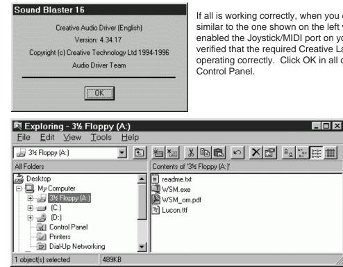
If all is working correctly, when you click on the "Settings" button, a dialog similar to the one shown on the left will appear. At this point, you have enabled the Joystick/MIDI port on your Sound Blaster 16 card and have verified that the required Creative Labs software driver is installed and operating correctly. Click OK in all open dialog boxes and close the Control Panel.
